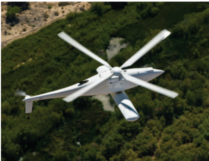
The Boeing Forester autonomous unmanned helicopter was designed to be quiet, hover, reach high altitudes, and travel great distances. (Boeing image.)
