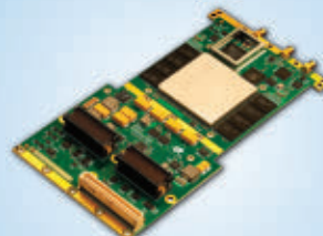
XPedite2400 Xilinx Virtex-7 FPGA-based XMC with high-throughput DAC
