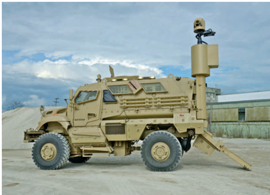
SELEX Galileo's Gyrocam 15-inch Triple Sensor (15TS) systems on an International MaxxPro Mine Resistant Ambush Protected (MRAP) vehicles, used by the Italian Army in coalition operations. The Gyrocam 15TS can be mast-mounted on virtually any land vehicle for remote surveillance needs.
