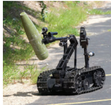
DARPA is using the QinetiQ TALON IV tracked UGV to carry a variety of sensor payloads as part of the Autonomous Mine Detection System (AMDS) to detect, mark, and neutralize explosive hazards.
